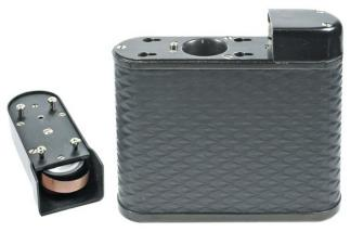
Tape cassette (left) and recorder. A 3V dry battery fitted into the hole in the centre.
